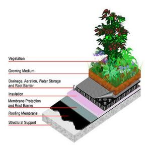
Figure 2.3: Layers of a Green Roof (LIDC, 2007)
